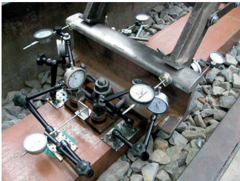
Repeated load test on the basis of DIN EN 13481-3
