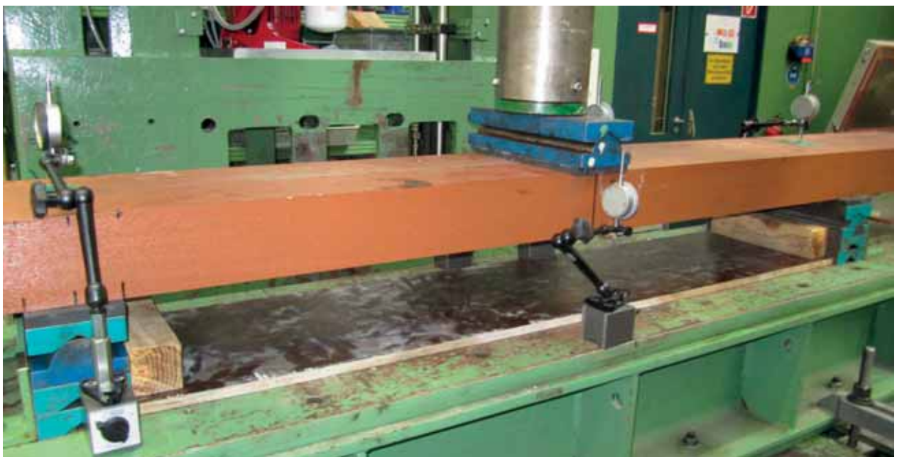
Fatigue test in sleeper centre (2.0 million load cycles)
