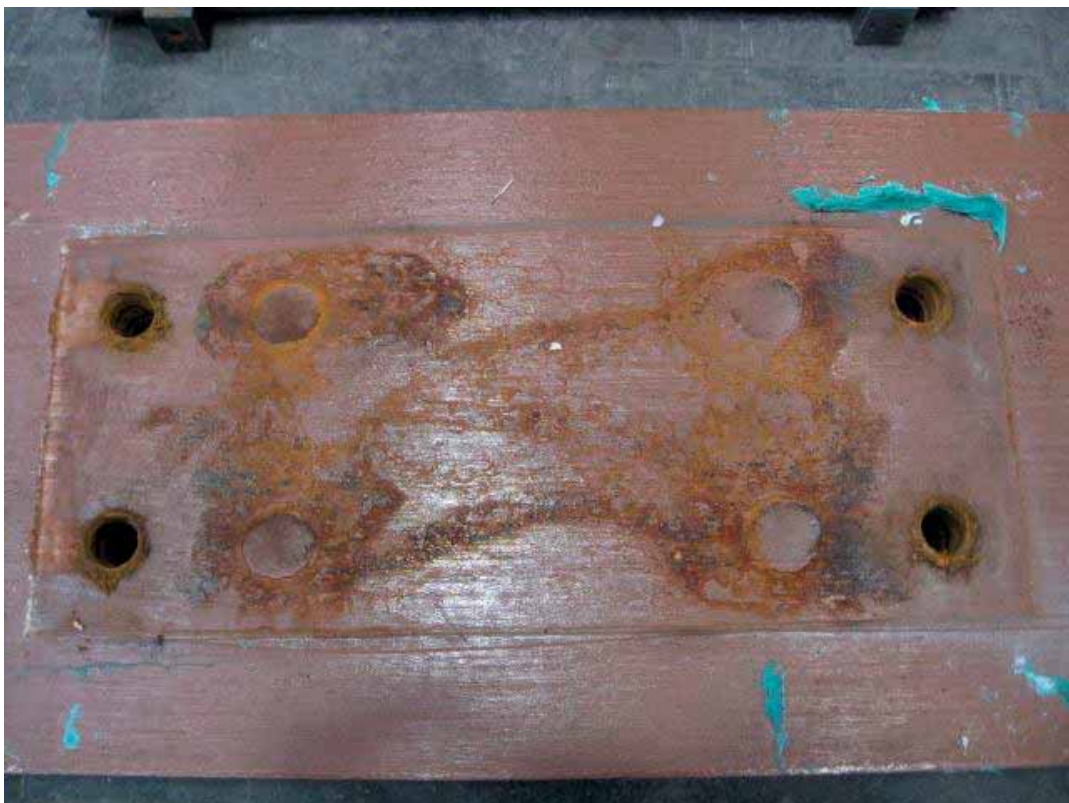
Slight plastic deformations of max. 0.23 mm at the sleeper surface following repeated load test (3.0 million load cycles)
