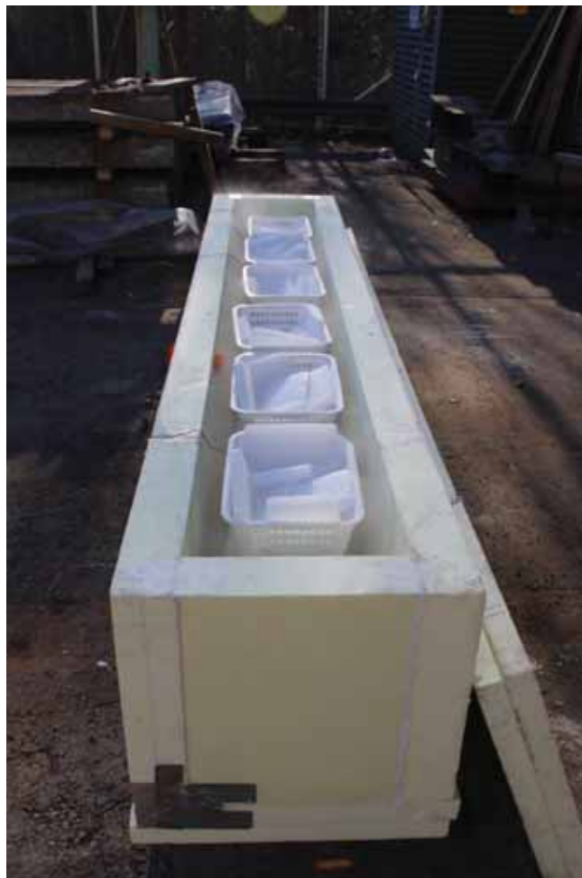
Figure 3 Cooling box. FFU sleeper on the bottom and dry ice in baskets on top of the sleeper.
